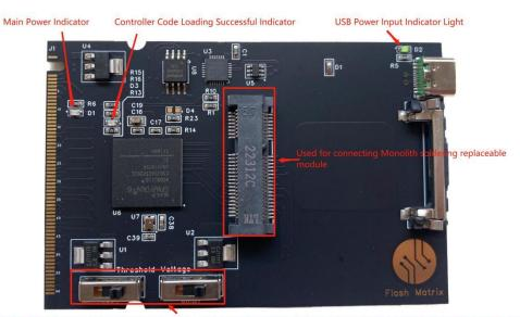
3-level adjustable signal level threshold switch. The switch on the left controls the Gold Finger, and the switch on the right controls the msata interface direction. Left: 1.8V, Middle: 3.3V, Right: 2.5V. The default configuration is 3.3V, which is the middle position
